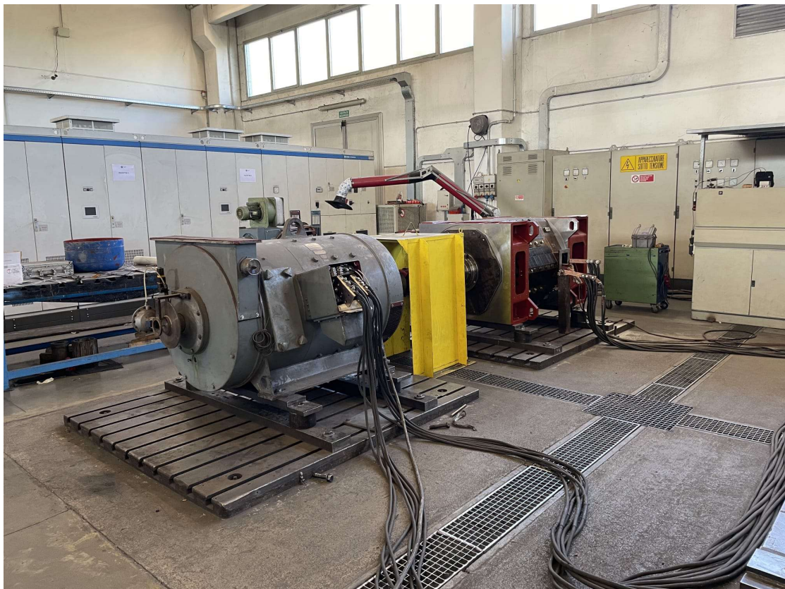
Figure 23: Load characteristic test of an in-house manufactured DC motor.
