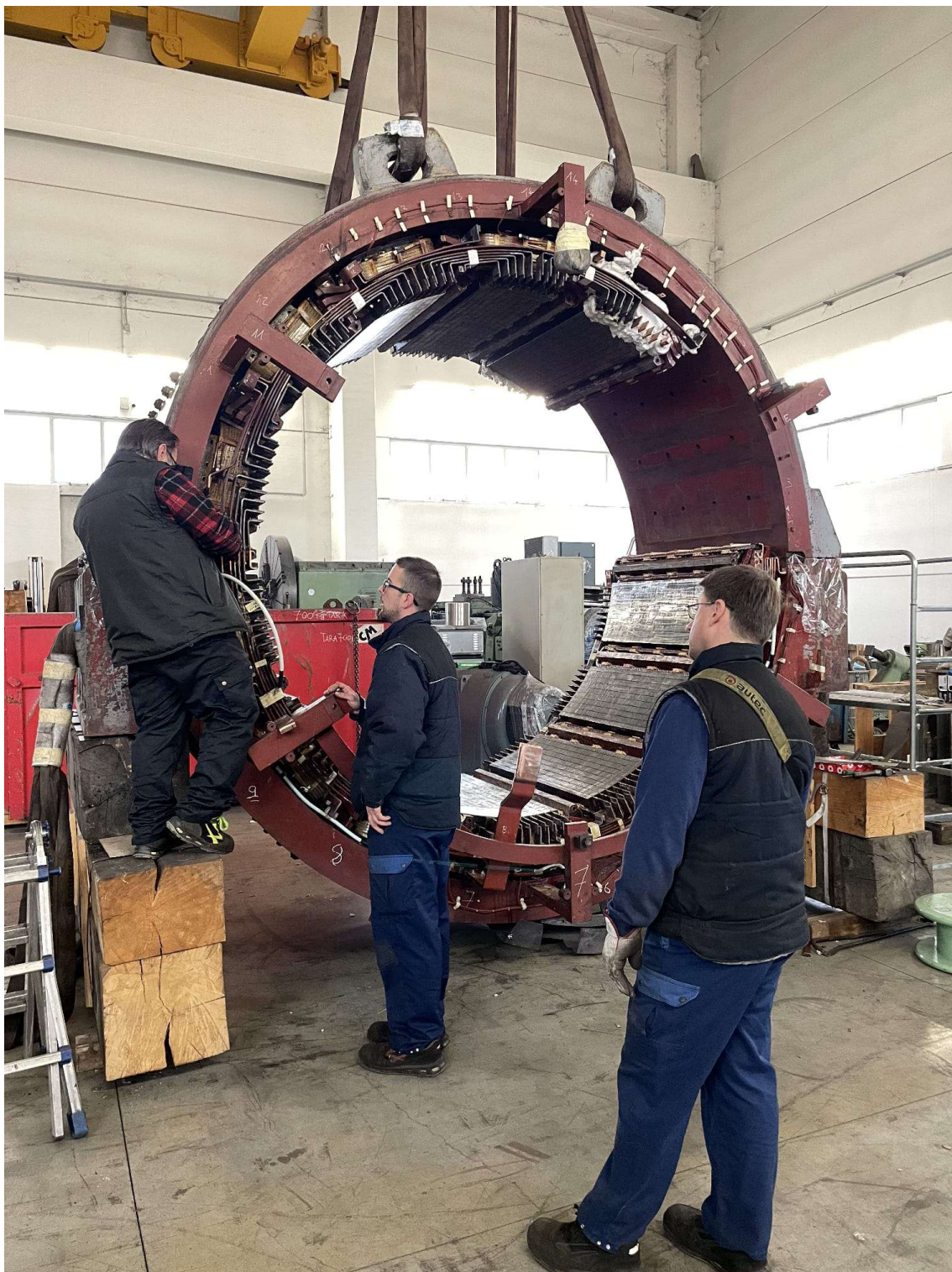
Figure 1: Overhaul and stator rewinding of an MCF motor, rated torque 555kNm.
