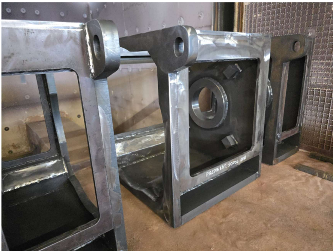
Figure 18: DC motor end closures undergoing stress-relief heat treatment.
