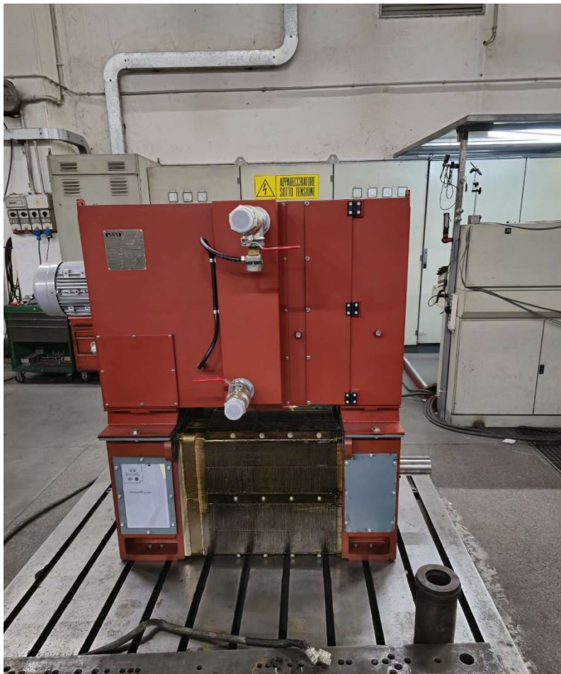
Figure 15: Frame 315 DC motor for rolling mill stand and roughing applications, 3,900 Nm.
