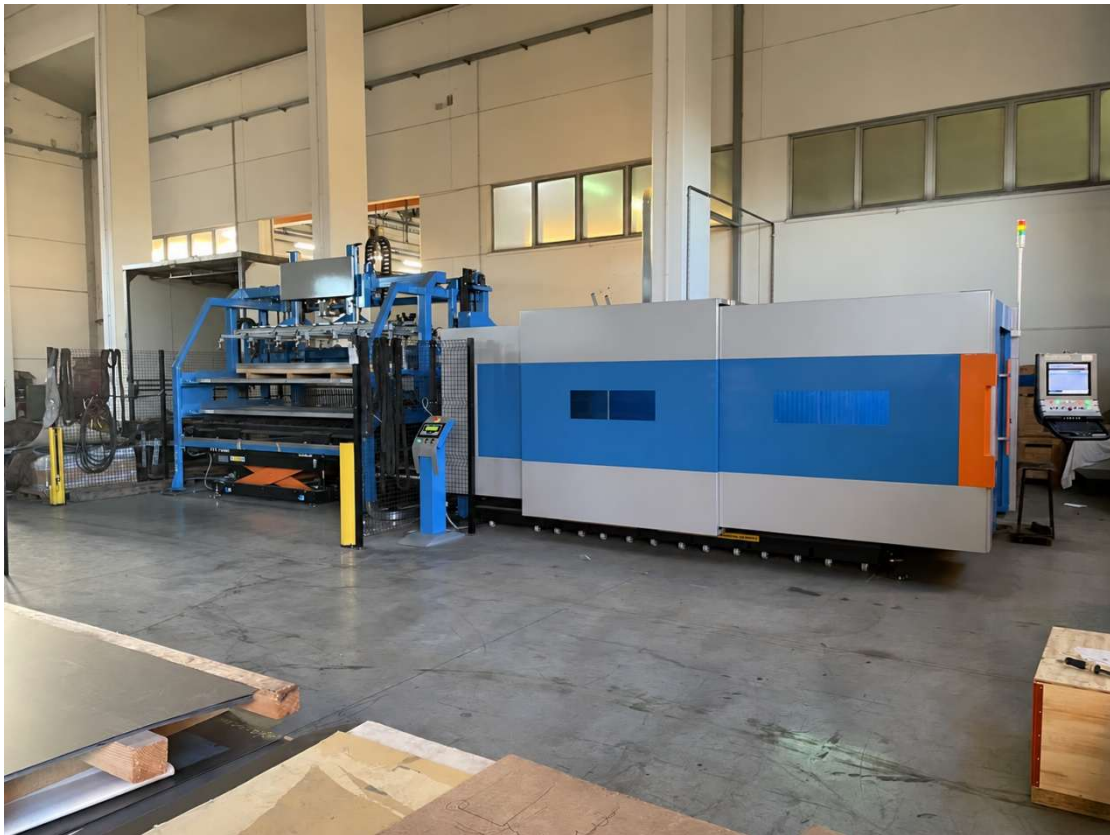
Figure 7: Laser Genius with compressed-air cutting technology.
