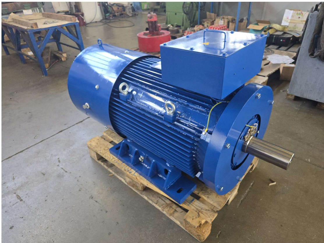
Figures 13 - 14: Special frame 355 AC motor for a cut-off saw, with welded steel frame and high-efficiency rectangular-wire winding (>95% actual efficiency).
