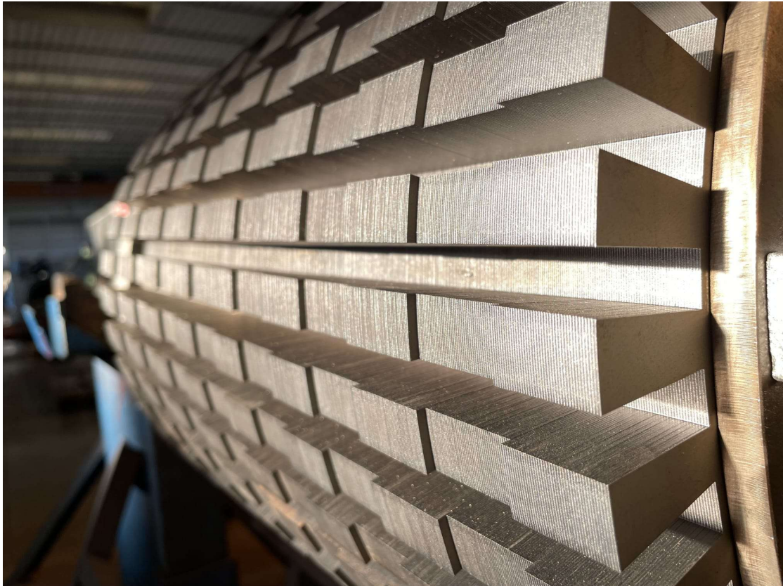
Figure 19: DC rotor core stacking.
