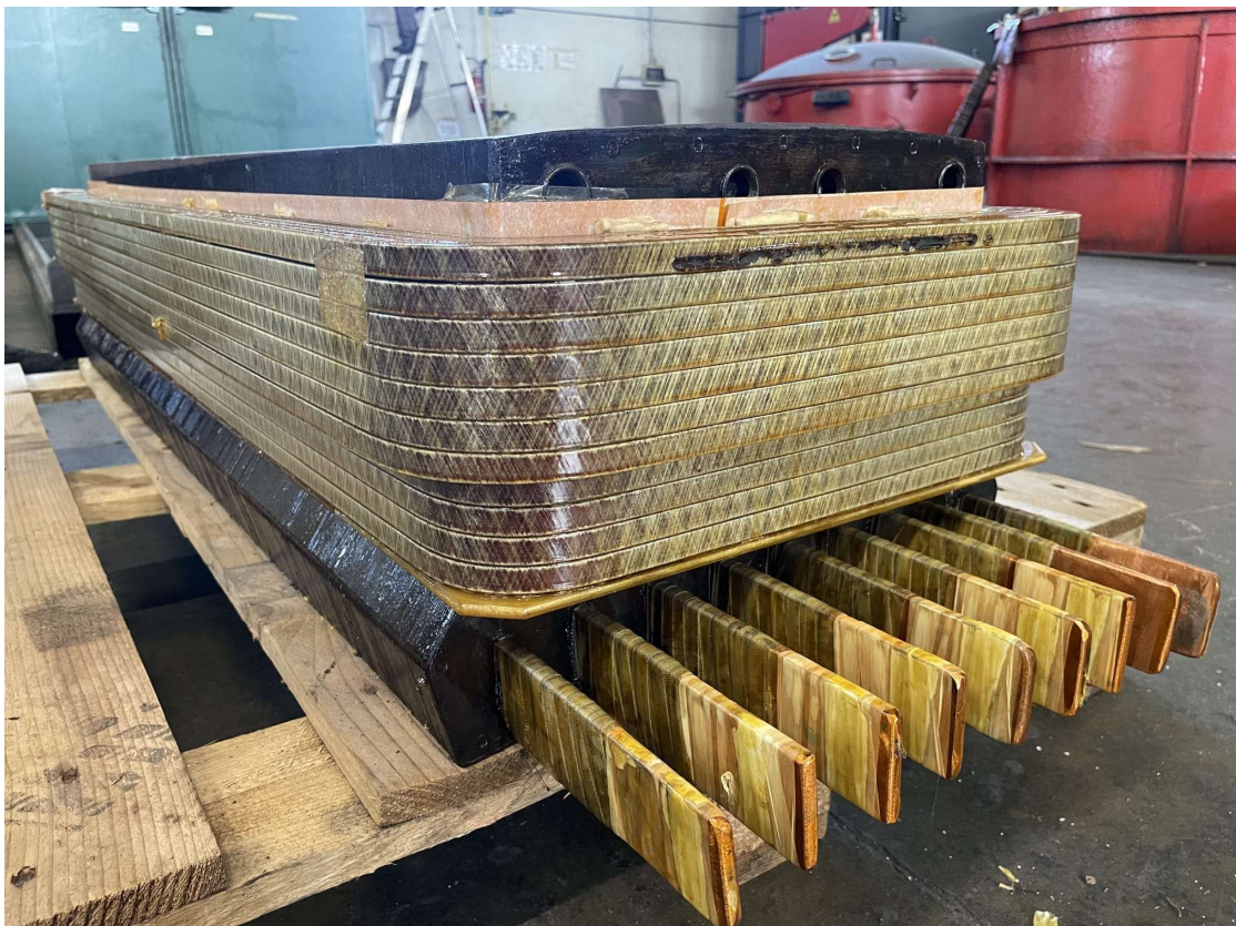
Figure 20: Reverse engineering and manufacture of a replacement main pole for an ASEA split-stator DC motor.
