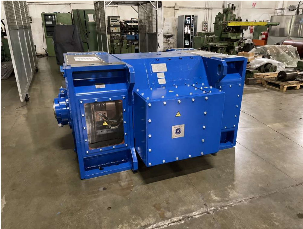
Figure 2: Design and manufacture of a frame size 500 DC motor for an extruder, torque 10,500 Nm.
