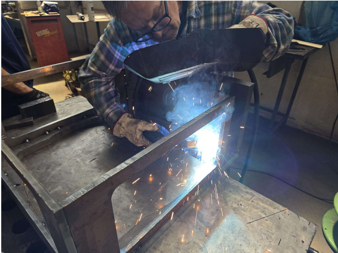
Figure 17: Manufacture of DC motor end closures.
