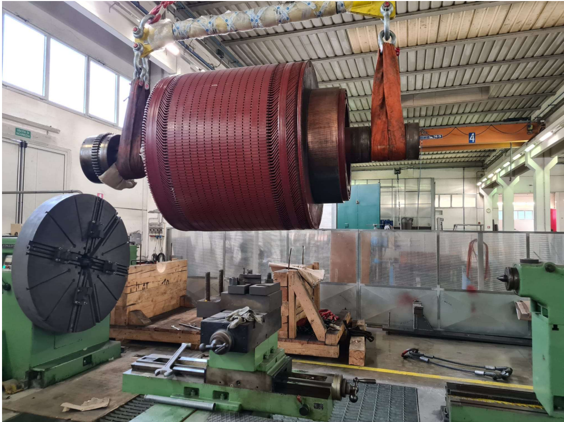
Figure 25: Overhaul of a Ge.Co. Westinghouse motor during a summer shutdown.
